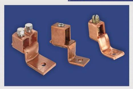
These are mechanical terminal lugs made from pure Copper and have a offset tongue and a hole for joining a wide range of cable to equipment pads or bar. They are easy to install with screwdriver or wrench. The connector is re-usable.
