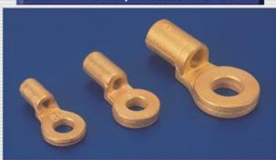
Brass Cast and Stamped Lugs for various electro-mechanical applications. They are mostly made to user specifications and used for battery cable harnesses. They are to be soldered or crimped with the battery cable.
