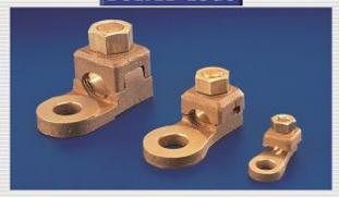
Bolted Copper alloy Lugs are a quick and easy way of making a connection on a normal or flexible conductor. Palms are machined top and bottom for bolTing on either surface. They can be reused multiple times. Barrels have internal corrugations in the clamp to assist with current transfer.
